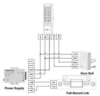
Connect to 12VDC power, red wire connect to positive (+), black wire connects to negative (-).
