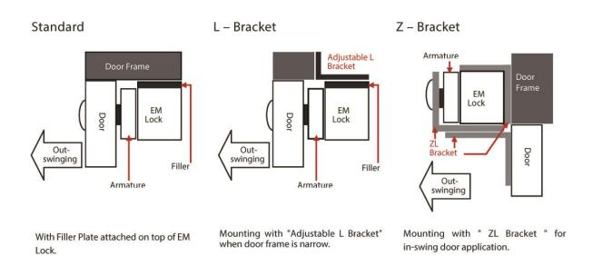
Mounting Procedure: Remove the original "Filler Plate" attached to the EM Lock, and replace with "Adjustable L Bracket" set.
