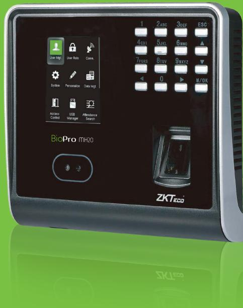
BioPro MH20 is the first ever Time & Attendance and Access Control Terminal to be associated with Z-ID Fingerprint Reader, Face Recognition and RFID Card (optional) functions. With the new Z-ID Fingerprint Reader, the operation remain stable under strong light source and high preciseness of verification of wet and rough fingers. With the innovative features, BioPro MH20 is bringing you the whole new experience.
